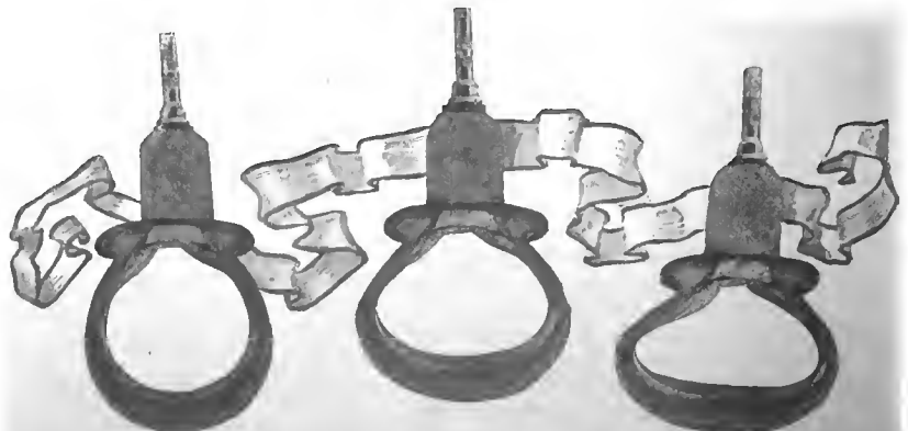
Fig. 2—Moderate deformation of well-inflated tire.
